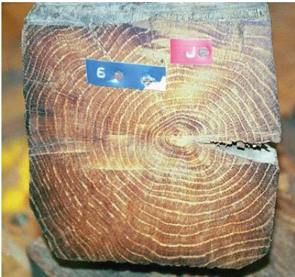
Figure 6.13 A boxed-heart post that has been in service for a long time, and has dried out. The member is sectioned to show the typical single main fissure passing to the heart
