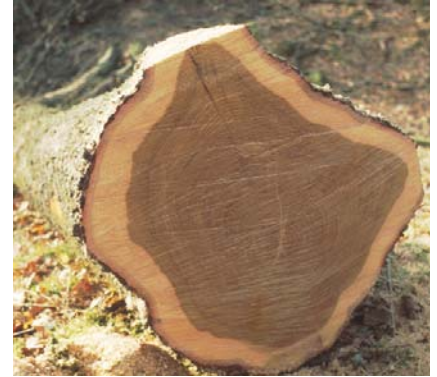
Figure 4.2 Oak log after felling showing clear differentiation between sapwood and heartwood.
