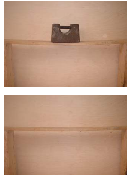
Figure 4.11 a, top: A plank of green oak, 100 mm wide by 20 mm deep, spanning 1.2 m with a central point load b, above: After six months the plank had dried out. With the load removed, a residual deflection of 19 mm remained
