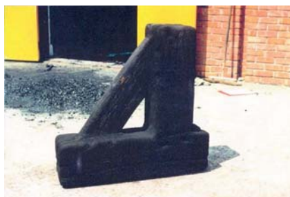
Figure 4.13 Charred oak. A Globe Theatre (see Case Study 9.1) joint after fire testing. The oak has suffered little charring; this is apparent as the shape of the elements is clearly defined. The assembly was subsequently successfully tested to verify its remaining strength Photo: Jon Greenfield
