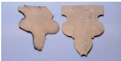
Figure 9.5.9 left: a section of original oak rib, which, before the fire, was some 350 mm deep. Drawing the trunk outline from the curvature of the growth rings indicates that it was around 1.5 m in diameter. right: a section of replacement oak rib made up of four laminations, 75 mm thick, grooved for loose tongues. They were kiln dried (which for this thickness took six months) and assembled with a urea formaldehyde adhesive (and the occasional bolt for peace of mind) Photo: P Ross
