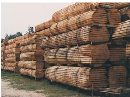
Figure 4.7 'Sticked and stacked' logs Photos: John Boddy Timber Ltd
