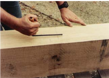
Figure 6.7 A grain scribe is being used to check slope of grain on the upper surface of the beam. The lateral surfaces may need to be checked in a similar way
