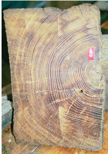
Figure 6.14 A sectioned halved beam taken out of service. The method of conversion was clearly as in Figure 6.12 b. The heart can be seen on the right-hand face. This is the “Fair Face,” having better appearance - showing few or no knots, and better resistance to exposure. Note the typical distortion of this type of member, similar to Figure 4.5 Sample B
