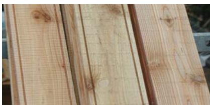
Figure 9.8.8 Locally-grown western red cedar cladding. Detail shows grooved boards with slots on the side away from the heart, so that cupping will occur outwards on the lower boards and downwards on the upper boards maintaining a tight weather envelope Photo: Weald and Downland Museum
