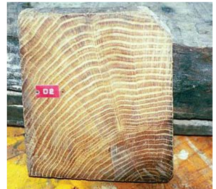
Figure 6.15 A quartered beam taken out of service. The method of conversion, usually for smaller posts, is clearly as shown in Figure 6.12 c. The heart can be seen in the bottom right-hand corner. Note the similarity of the drying distortion to Figure 4.5 Sample A
