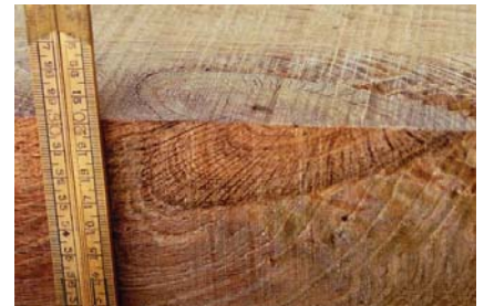
Figure 6.10 This heart-shaped feature on the edge of a beam is termed an arris knot. It has a “root,” like that of a molar tooth, penetrating right into the section. Simplified views of two arris knots are also shown in Figure 6.8, but that Figure is more typical of a small softwood member. Because of the deep disturbance to the longitudinal grain, and the emergence of the arris knot amongst the extreme fibres of a beam, it is treated more strictly than the centre knot in Figure 6.17
