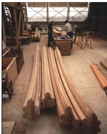
Figure 9.5.10 Assembled ribs, some six metres long Photo: P Ross
