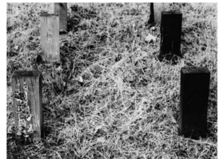
Figure 4.8 'Graveyard' tests Photo: © BRE
