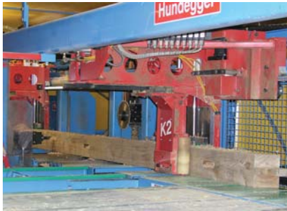
Figure 6.4 Hundegger numerically controlled CAD - CAM system in use for green oak framing manufacture Photo: T J Crump Oakwrights
